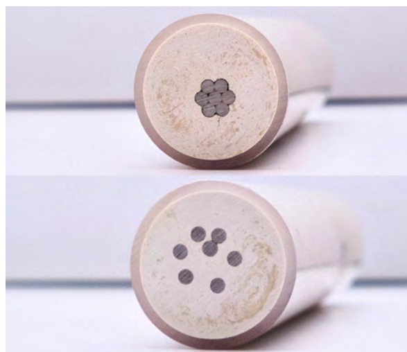
Cross section of a grouted cable bolt
